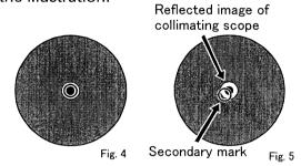
Focus the secondary, viewing into the collimating scope. Refer to the fig 4.
