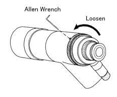
4. With an Allen wrench provided, turn the three adjusting screws and place the star exactly at the center of the crosshairs. Then, fasten the lock ring firmly to set the visual back in place. Then check the main tube to see if the star is still centered in the field of view of the ocular.
