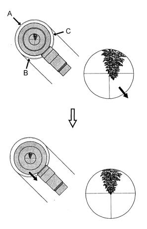
turned on. Turning it further in the clockwise direction brightens the illumination. Conversely, turning the knob counter-clockwise will dim illumination until it is switched off with a clicking sound. Refer to the illustration. Adjust the brightness of the illumination so as to see the star and the reticle at the same time at the lowest possible illumination level.
