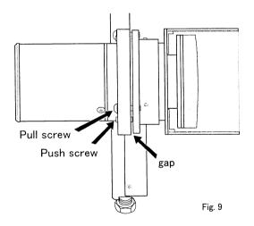
not only by using a pair of screws in a place, but by using the other pair of screws. In the Fig. 7, loosen the No. 3 pushing screw and tighten the pulling screw. When the mark approach half-way the center, loosen No.1 and 2 pulling screws, and tighten push screws. This means the optical adjustment for the secondary can be made by using all three pairs of screws.
