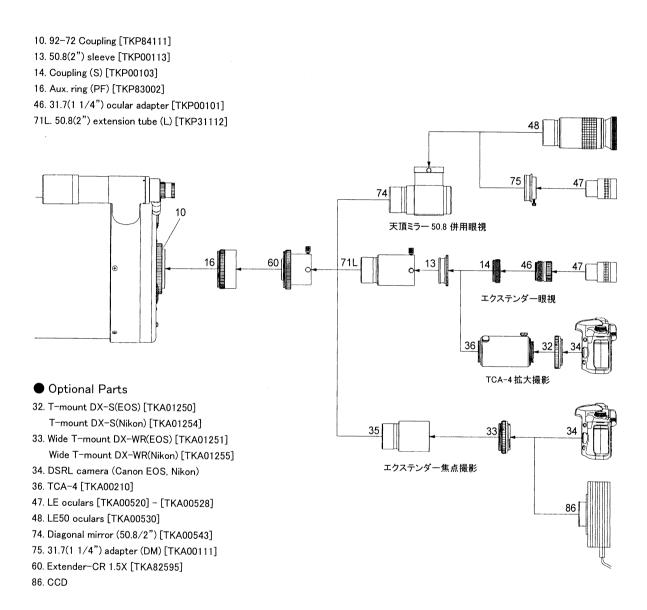
Note: Some 35mm DSLR cameras cannot be attached to T-rings or to Wide T-rings.
